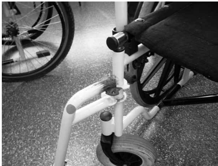
Figure 3: Example of a footrest swing away mechanism repaired by welding the footrest to the WC frame
